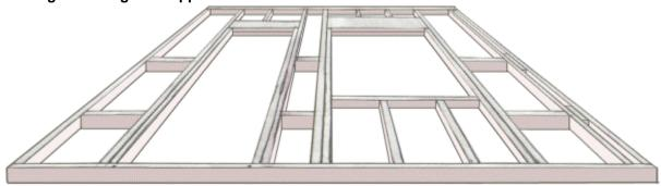
Just the Cripple Studs to go, which are the short Studs between the Header / Lintel and a Top Plate or between the sill and Bottom Plate.
