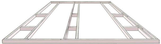
Fix the Noggings and Blocking in place between the Studs. At least one row of Noggings can help minimize twisting and warping.
