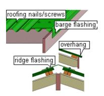
Ridge Capping and Barge Flashing Standard Ridge Capping is about 130 (5") each side of the apex, but can vary and any size can be made to order. Have the Ridge Flashing in mind when positioning the top Purlin. Fix to the Purlin at every second corrugation.
