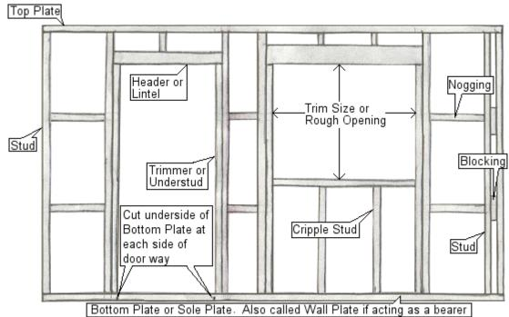
Wall Framing, excepting headers, is usually of 100x50 (2x4) stock, for perimeter or bearing walls. Internal non-load bearing walls can be of 75x50 (3x2) stock.
