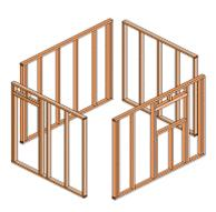
Make the Wall Frames up on even ground, referring to the 'Wall Frame and Stud Placement' Plan which shows the placement of the studs from a bird's eyeview. In this particular plan, the Studs are spaced at 600 [2ft] crs or o.c.(which means "at centers" or "on center"). This means the Studs are spaced apart 600 (2ft) from the center of one Stud, to the center of the adjoining Stud (where possible).
