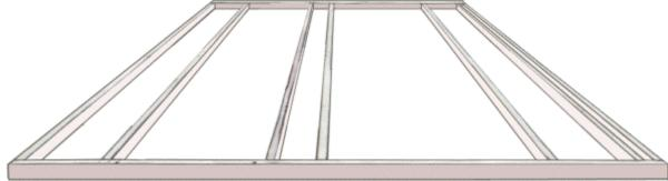
The length of the Stud should be the required ceiling height less the thickness of the Top and Bottom Plates as well as the thickness of the ceiling lining as well as a bit to play with, say 10mm (3/8").
